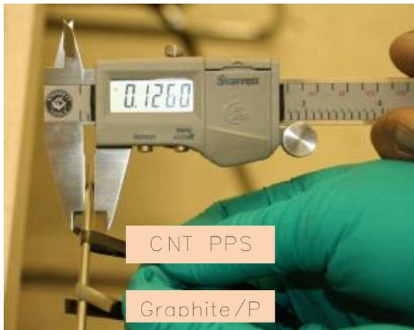
Figure 3 An example of Graphite PEEK based tape ‘failing’ around a small bend radius compared with a CNT PPS based tape. Both tapes have about the same chord modulus, thickness, and breaking strength.
