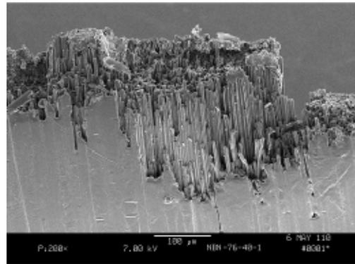
Figure 4. An SEM micrograph at 7 keV of graphite Peek composite fractured as in Figure 3.
