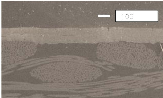
Figure 2. A prepregged CNT sheet bonded during fabrication to ordinary graphite composite. This geometry imparts extraordinary electric properties to the composite.
