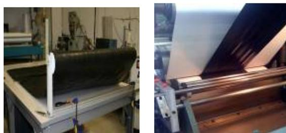
**Figure 1** (a) A 25 foot long CNT sheet and (b) a commercial prepregger infiltrating a 200 foot long DWCNT roll.
