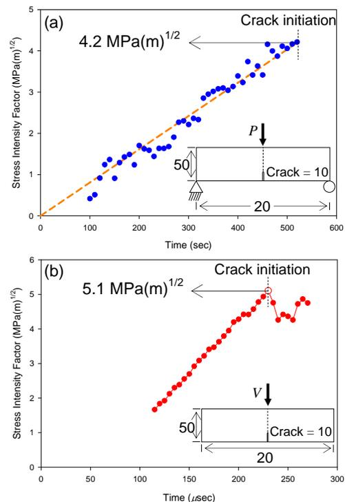
Figure 2. Measured stress intensity factor history of neat PETI-5 under (a) quasi-static loading and (b) impact loading: Inset indicates geometry of a specimen used in the respective test (units in mm).
