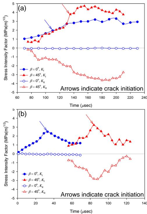
Figure 3. Mode-I and -II stress intensity factor histories for two fiber orientation angles: (a) IM7/PETI-5, (b) T800/3200-2 [5].
