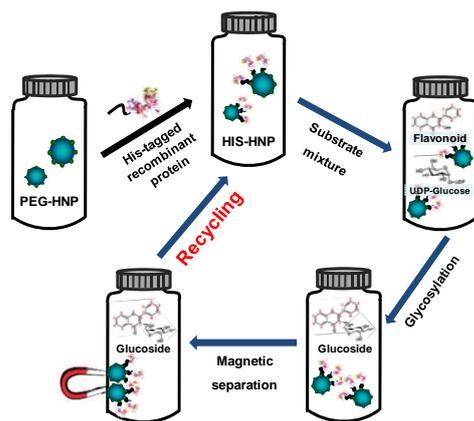
Fig. 1 Nano-immobilization of recombinant OleD GT on magnetic nanoparticle based on the affinity between his-tag and Fe<sub>3</sub>O<sub>4</sub>/silica/NiO nanoparticles, and its application to repetitive glycosylation of flavonoids.
