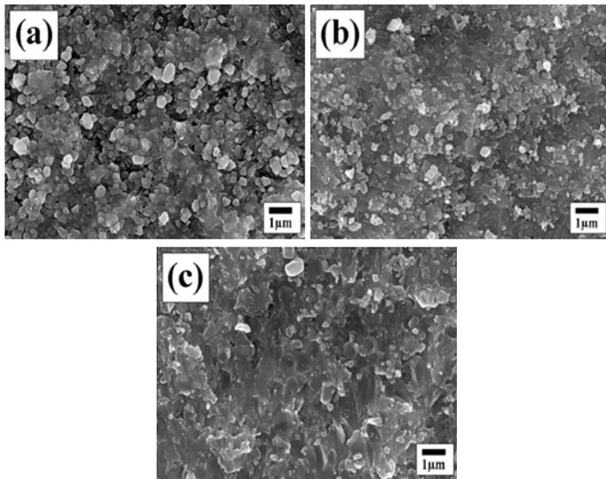
Fig. 2 FE-SEM micrographs of HA thin films at incident angles of (a) 0°, (b) 45°, and (c) 60°.
