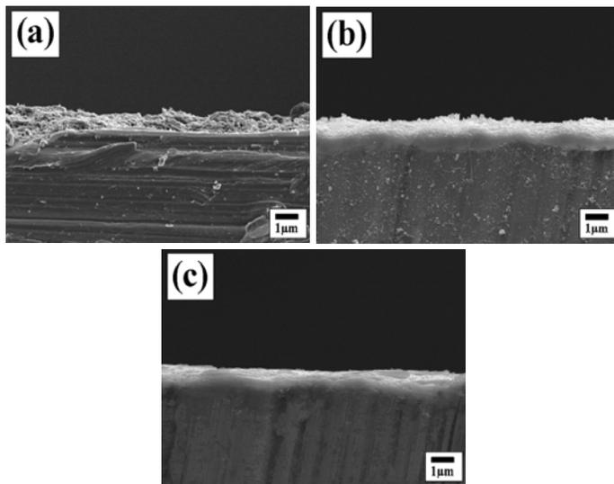
Fig. 3 FE-SEM micrographs of HA thin films formed at incident angles of at (a) 0°, (b) 45°, and (c) 60° cross-section.
