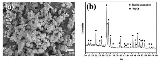
Fig. 1 FE-SEM micrograph and XRD pattern of bovine bone-derived HA powder.
