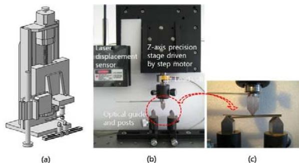
Fig. 3 Experimental device for 3-point bending test; (a) Schematic diagram, (b) Actual experimental device
