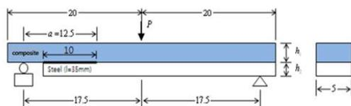
Fig. 1 Shape of SLB (single-leg bending) specimen
