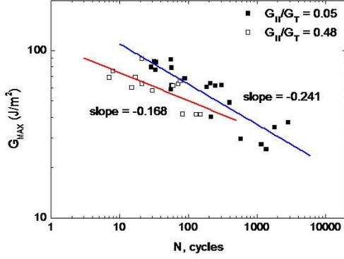
Fig. 4  $G_{MAX}$ -N (onset of crack growth) curves
