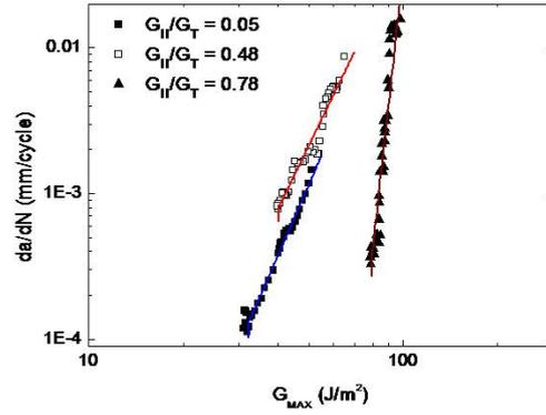
Fig. 5 Crack propagation rate- $G_{MAX}$  curves
