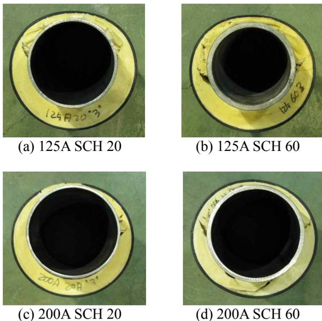
Fig. 3 Specimens after compressive loading experiment
