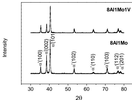
Fig. 2. XRD patterns of hot-rolled Ti-8Al-1Mo and Ti-8Al-1Mo-1V alloys.
