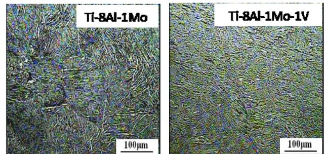
Fig. 4. Optical micrographs of hot-rolled Ti-8Al-1Mo and Ti-8Al-1Mo-1V alloys
