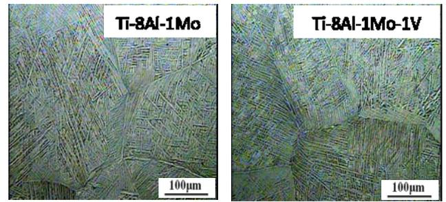
Fig. 3. Optical micrographs of as-cast Ti-8Al-1Mo and Ti-8Al-1Mo-1V alloys
