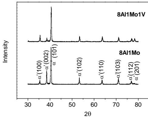
Fig. 1. XRD patterns of as-cast Ti-8Al-1Mo and Ti-8Al-1Mo-1V alloys.
