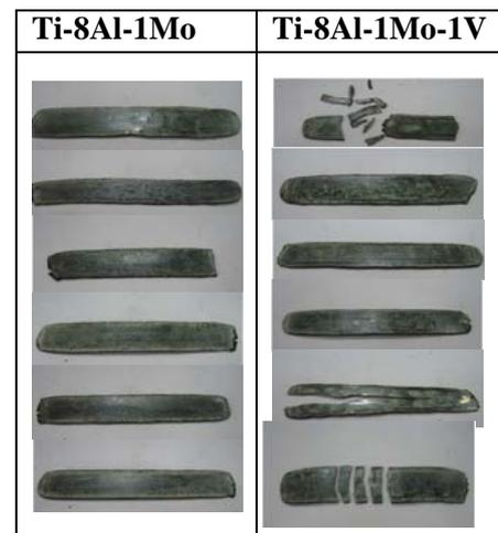
Fig. 5. Hot-rolled samples of Ti-8Al-1Mo and Ti-8Al-1Mo-1V alloys
