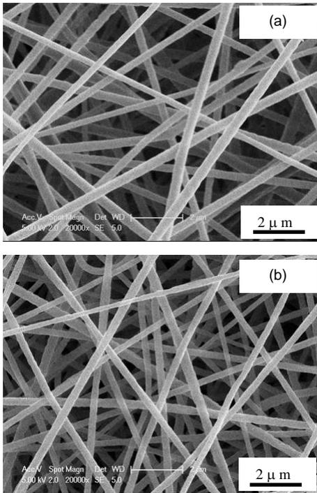
Fig. 1 SEM observations of electrospun fibres of (a) pure PLA mat and (b) PLA composite mats containing 7.5 wt.% cellulose whiskers.
