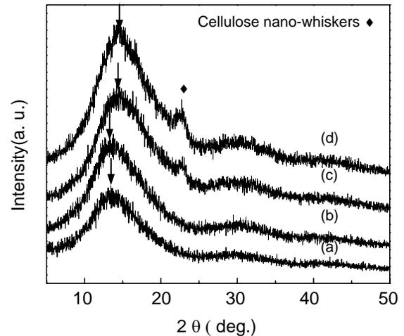
Fig. 3 X-ray diffraction patterns of (a) pure PLA, and PLA with (b) 2.5 wt.%, (c) 5.0 wt.% and (d) 7.5 wt.% cellulose nano-whisker composite mats.
