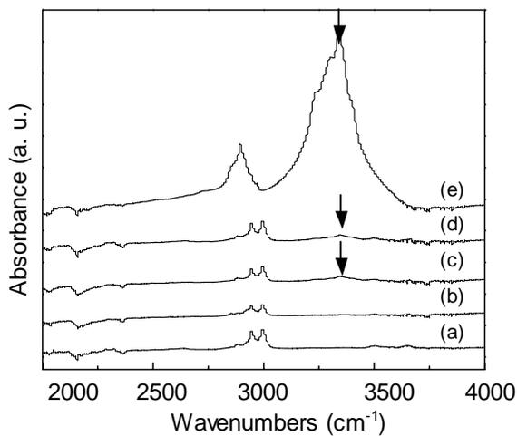
Fig. 2 FTIR spectra of (a) pure PLA, and PLA with (b) 2.5 wt.%, (c) 5.0 wt.% and (d) 7.5 wt.% cellulose nano-whisker composite mats, and (e) BC nano-cellulose whiskers.
