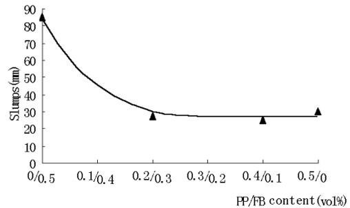
Fig.1 Influence of PP/FB content to concrete slumps
