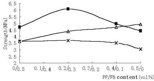
Fig. 3 Effects of PP/FB content to flexural and splitting tensile strengths of concrete, ×-7d flexural; ■-28d flexural; △-28d splitting tensile.
