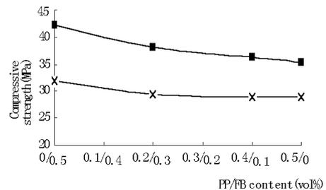
Fig.2 Effects of PP/FB content to compressive strength of concrete, ×:7d; ■:28d.
