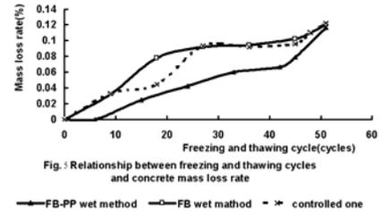
Fig. 5 Relationship between freezing and thawing cycles and concrete mass loss rate
