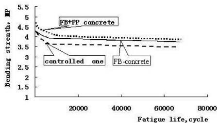
Fig.4 Relationship between bending fatigue life and bending stress
