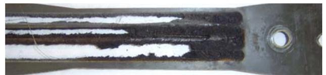
Fig. 4. Burnt of the CFRP epoxy matrix, due to the bad cutting of worn tools, after 42 mm of the slotting operation.
