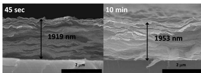
**Fig. 1.** Representative cross-sectional SEM images of {MMT-(sol-gel ZrO<sub>2</sub>)<sub>30</sub>} multilayer synthesized (Holding time in air are labeled). See Ref. 5 for more details.
