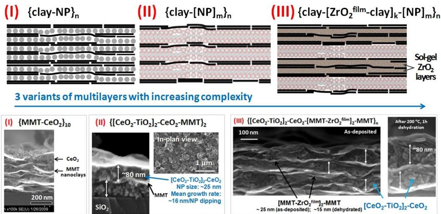
Fig. 2: Three variants of the targeted multilayers and representative SEM images.
