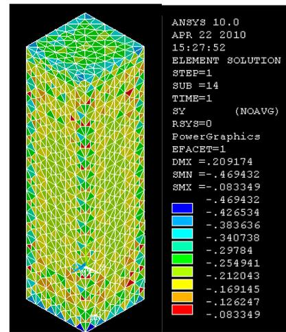
Fig.5. Normal stresses at failure load in steel plates.
