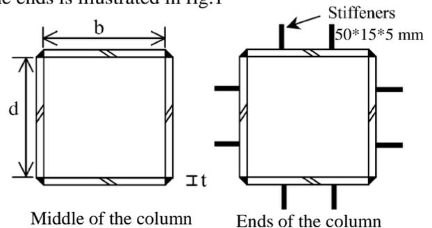
Fig.1. Short column cross section [1].
