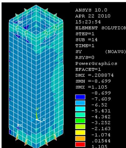
Fig.4. Normal stresses at failure load in steel plates.
