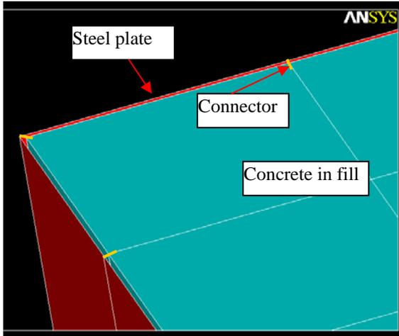
Fig.3. Connection between the steel plate and the infill concrete.
