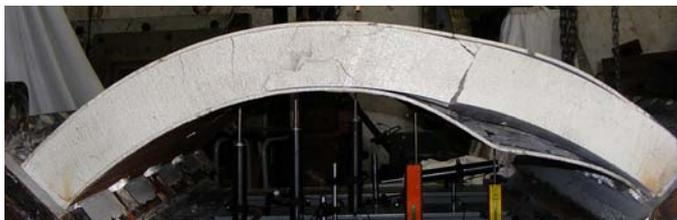
Figure 3. Plain SCS sandwich failure at ultimate load
