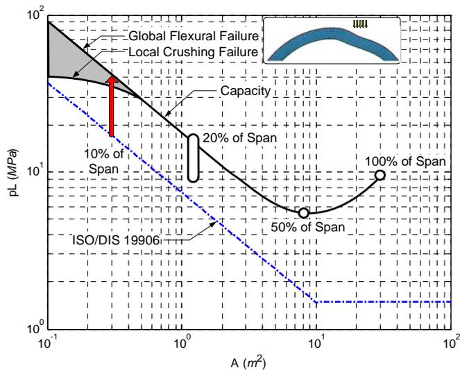
Figure 2. Analytical strength versus patch dimension (prototype scale)
