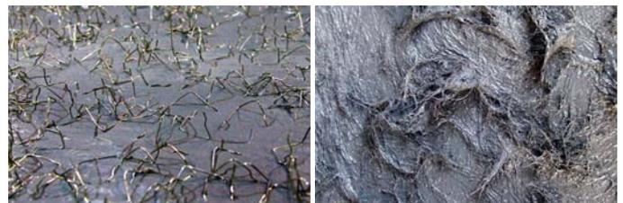
Figure 4. Prepared surface with epoxy and fibers
