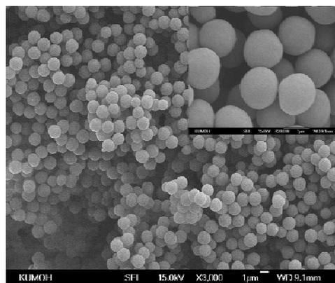
Figure 1. Silica particles.
