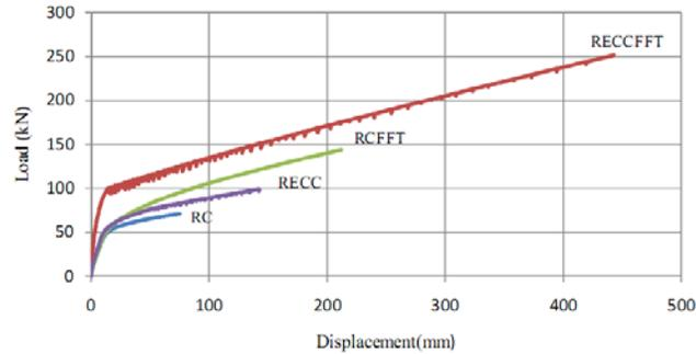
Figure 1 Effects of ECC and FRP tube
