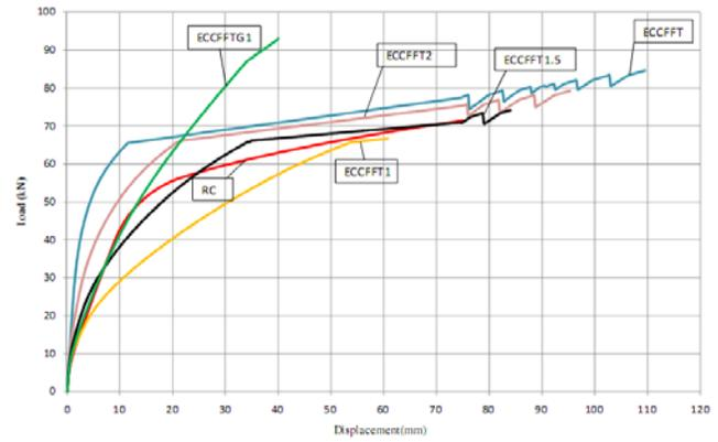
Figure 3 Effects of ECC length and FRP Tube
