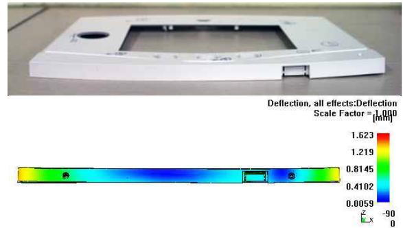
Fig. 2 Comparison between the deformation of actual product and analysis result
