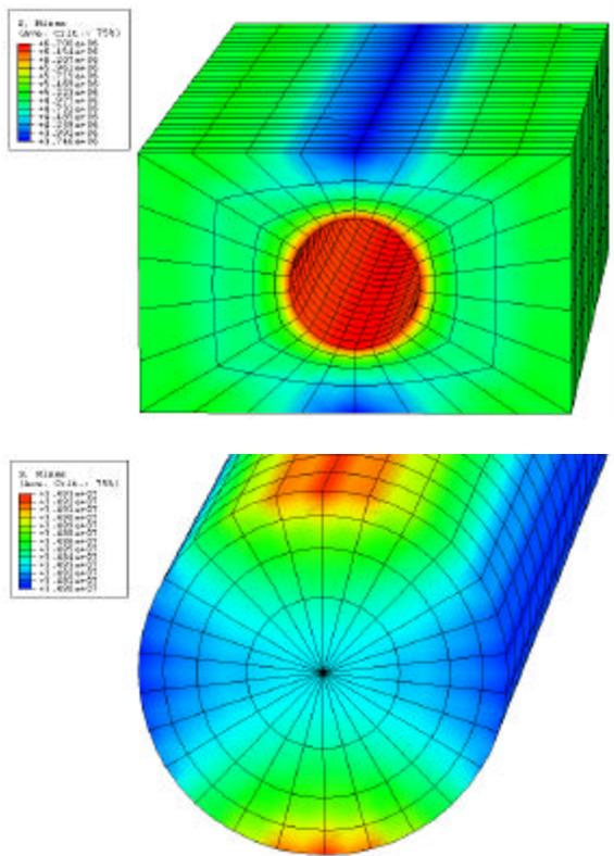
**Figure 1** Residual stresses of the Cu matrix and the Ag fibers and the Cu matrix after application of a load
