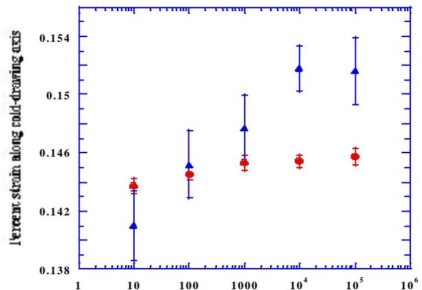
**Figure 2** Development of the longitudinal percent strain of Cu (circles) and Ag (triangles) in Cu/25%Ag composites as a function of cyclic loading to 20% of the elastic limit.
