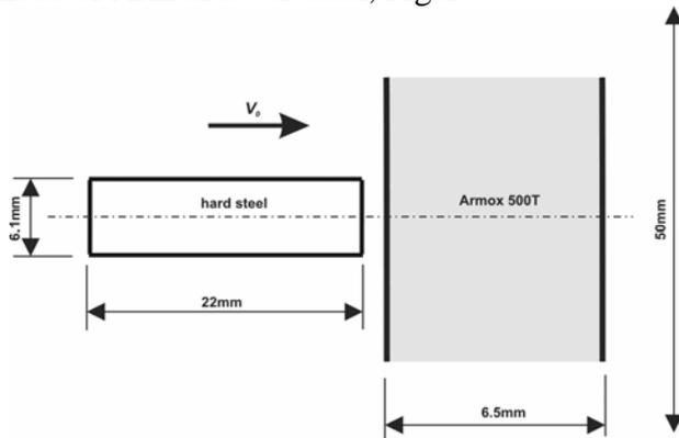
**Fig. 2.** Dimensions of the target disc and the cylindrical impactor.
