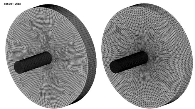
**Fig. 3.** The impactor and target mesh overview for hex (a), and tetra (b), mesh topology.
