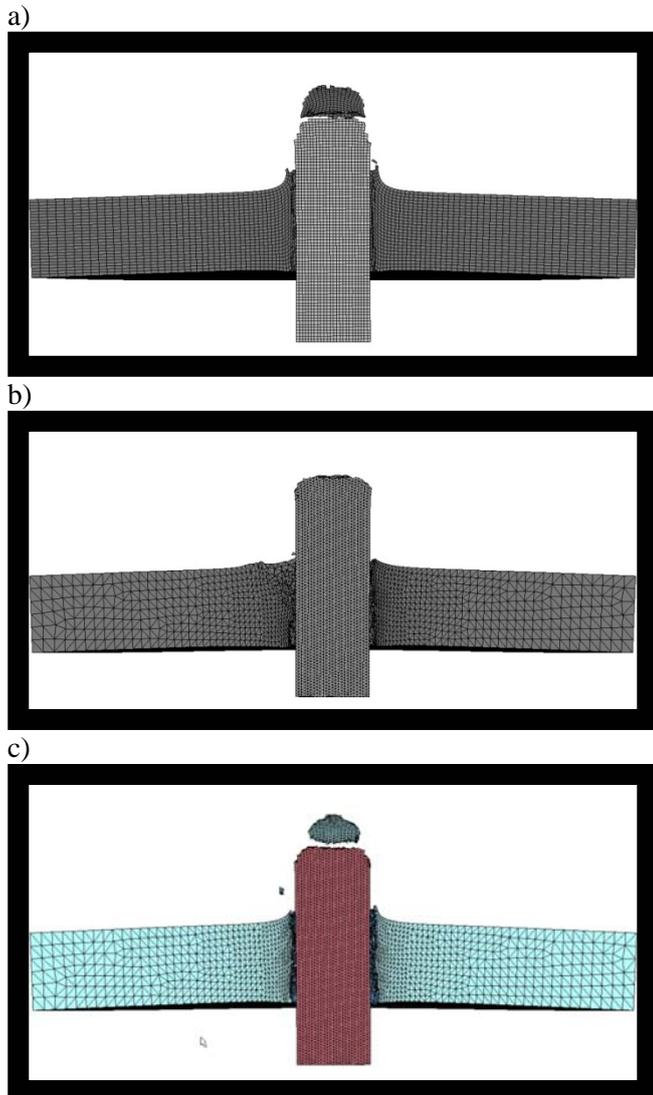
**Fig. 4.** A comparison of the computer simulation results for three cases at 30th microsecond after impact: (a) FEM method with hex mesh topology, (b) FEM with tetra mesh, (c) EFG method with tetra mesh.
