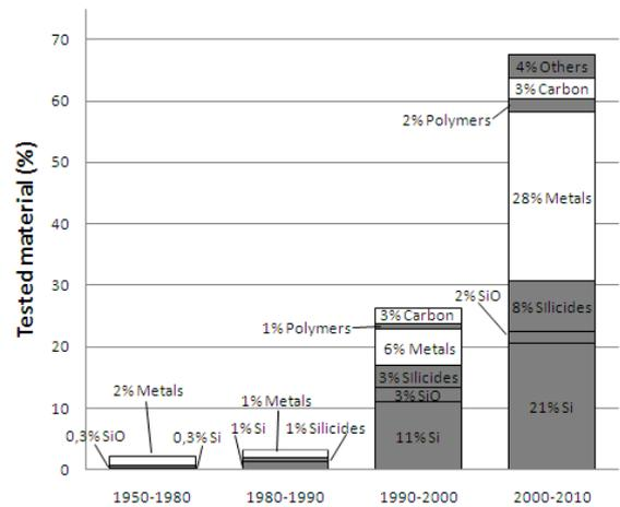
Figure 4 Materials tested at micro and nano-scale.
