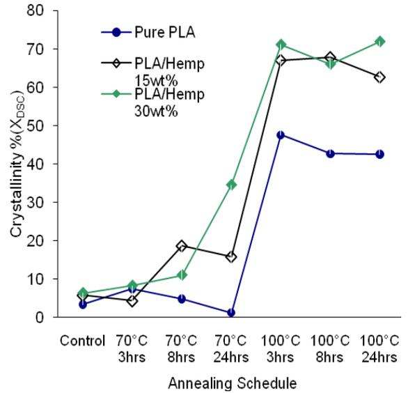
**Figure 6. PLA crystallinity for different annealing treatments**
