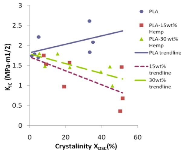
**Figure 7.  $K_{Ic}$  versus crystallinity isolated from fibre content for alkali treated fibre composites.**
