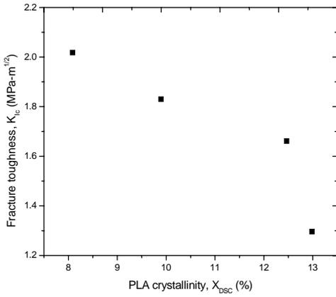
**Figure 4. Relationship between  $K_{Ic}$  and crystallinity for PLA and composites of different fibre contents.**
