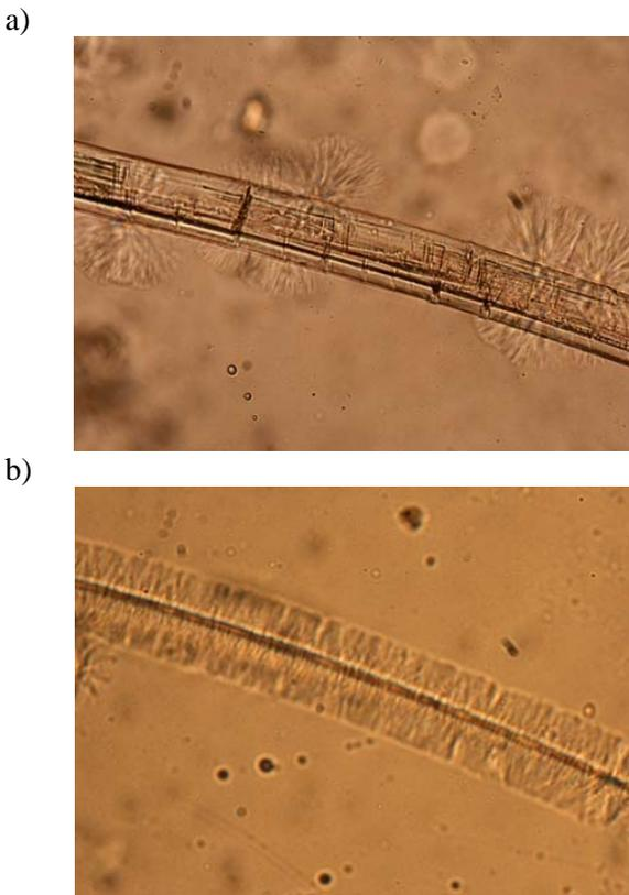
**Figure 5. Transcrystalline layer of PLA with a) untreated and b) treated hemp fibre surfaces.**
