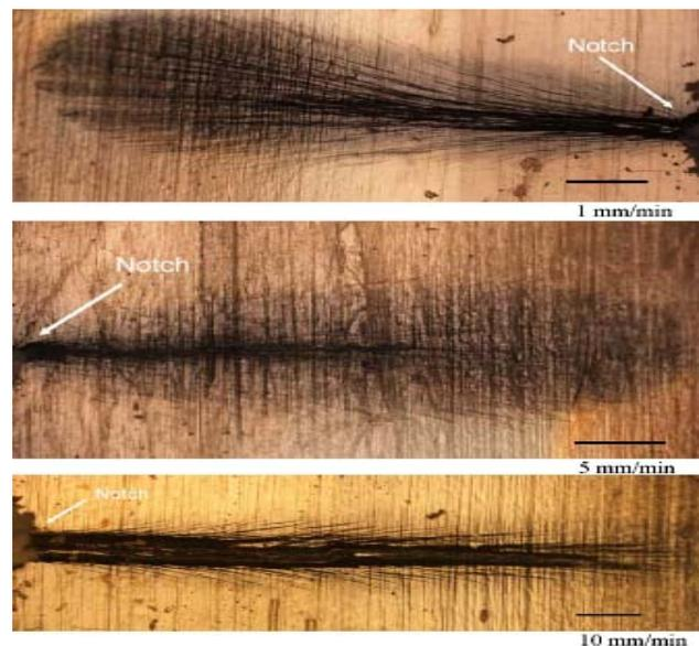
Figure 2. Light micrographs of crazing in PLA during fracture toughness.
