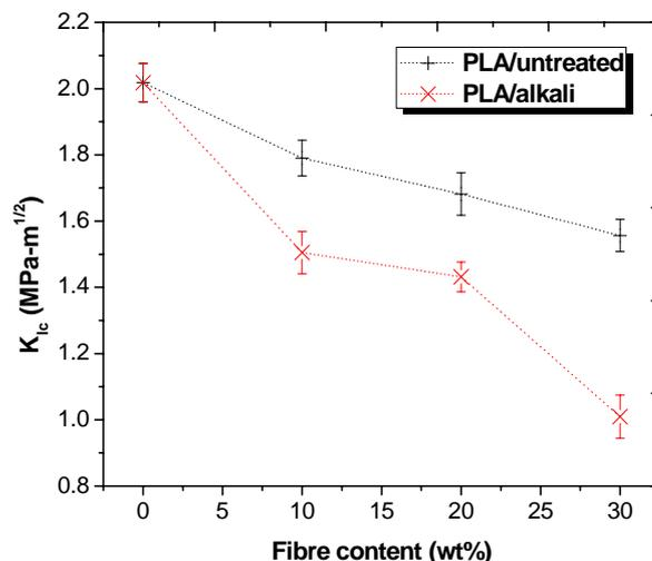
Figure 3.  $K_{Ic}$  versus fibre content for untreated and alkali treated fibre.
