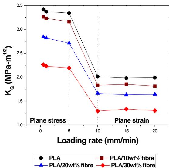
Figure 1.  $K_Q$  as a function of loading rate at different fibre contents.
