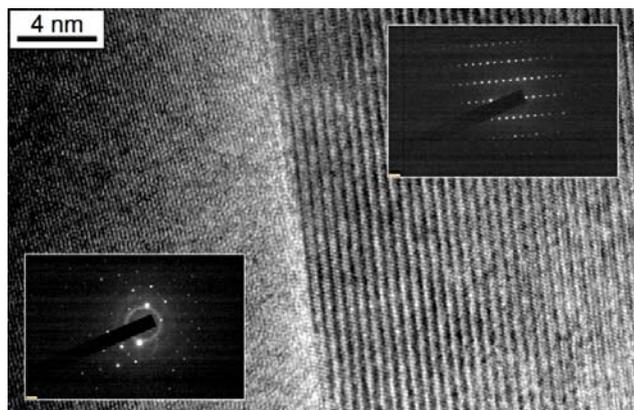
Fig.1. High-resolution TEM micrograph of a grain-boundary region from the sample  $Gd_5Ge_2Si_{2-y}Fe_0y$  ( $Y = 0.25$ ) and the corresponding electron-diffraction patterns.
