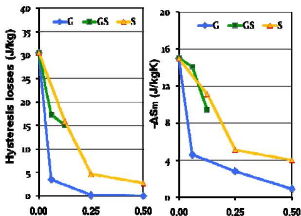
Fig.2. Dependence of the hysteresis losses and entropy change of the amount of Fe addition and the mechanism of substitution.
