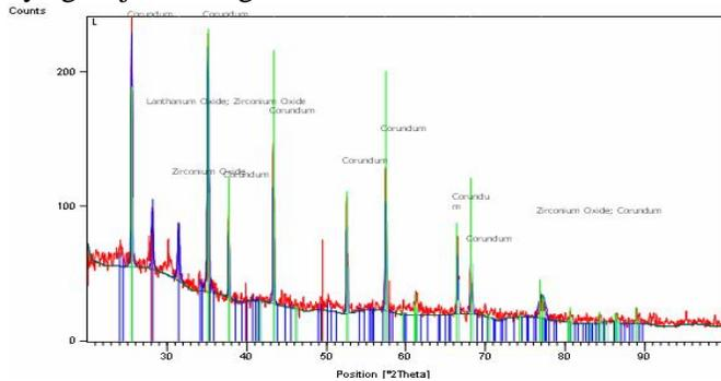
Fig 4: XRD pattern of lanthanum oxide based zirconia by agate jar method
