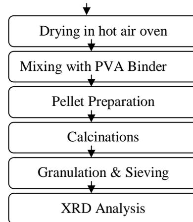
Fig1: Flow chart for  $La_2Zr_2O_7$  Powder Preparation by Wet Ball method.
