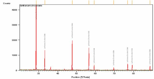
Fig 5: XRD pattern of Lanthanum oxide based Zirconia
