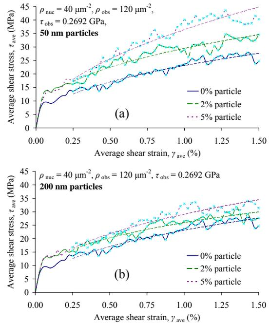
Fig. 2. Mean overall response of composite material for different particle volume fraction with uniform particle size of (a) 50, and (b) 200 nm.
