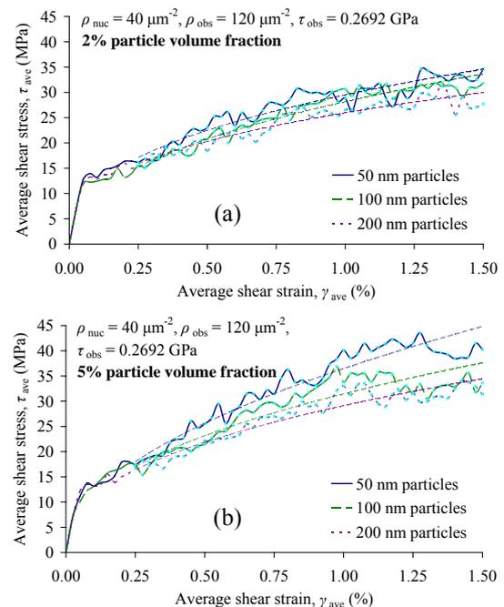
Fig. 3. Mean overall response of composite material for different uniform particle size with particle volume fraction of (a) 2, and (b) 5 per cent.
