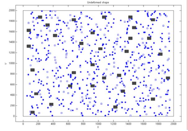
Fig. 1. 2D unit cell model showing the locations of the particles (shaded boxes), dislocation sources (white rectangular markers) and impurities represented by point obstacles (small dark spots).
