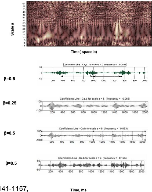
Fig. 3 Wavelet analysis of torsional acceleration for faulty (cracked) gear using optimized wavelet filter
