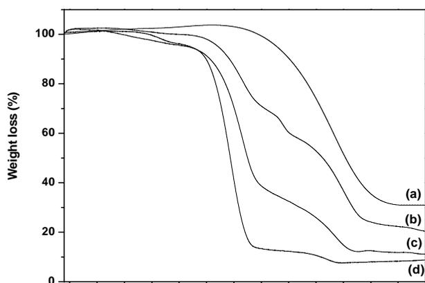
**Figure 3.** TGA of cured samples (a) PB-100/PER-0 (pure cured PB), (b) PB-80/PER-20, (c) PB-20/PER-80, (d) PB-0/PER-100 (Pure cured PER).
