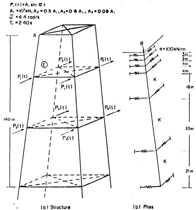
Fig. 1. Simple space frame characteristics.
