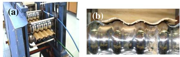
Fig.2 Continuous rollforming of corrugations (a) Woodfibre-PP (b) Wood veneer
