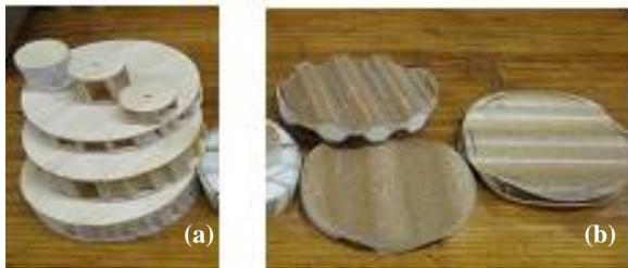
Fig.3 Sandwich panel specimens for impedance tube test (a) Out-of-plane scheme (b) In-plane scheme
