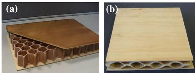
Fig.1 Hollow core panels (a) Woodfibre-PP core (b) Double corrugation wood veneer core
