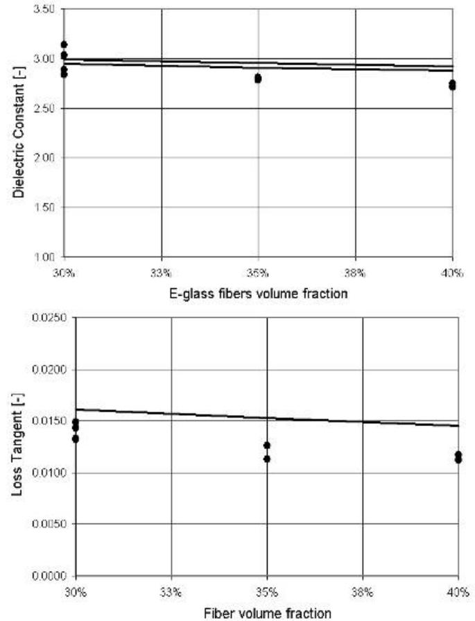
Fig 2. Effective dielectric constant and loss tangent for composite system at 100 KHz
