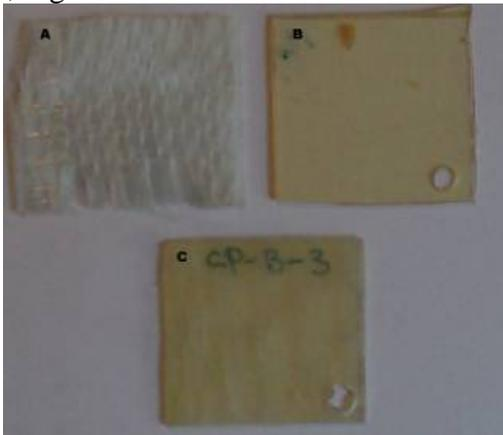
Fig. 1 DER 324/E-glass composite samples
