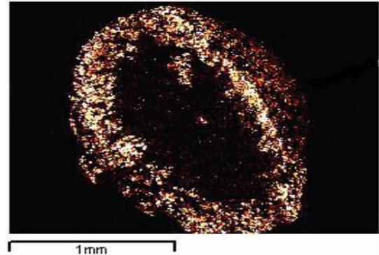
Figure 2. EDX image of metallic particles from TLPS surrounding a carbon fiber tow bundle
