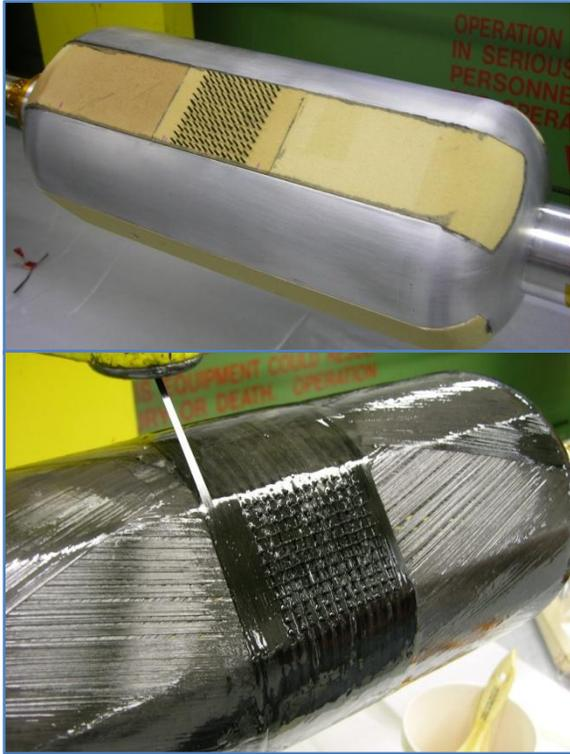
Figure 1. Filament winding over high-conductivity Z-pins. Bare mandrel with Z-pins inserted into foam blocks (top). Winding carbon fiber over Z-pins (bottom).
