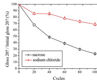
Fig.1 Gloss/initial gloss(%) at  $20^\circ$  during Taber Test.
