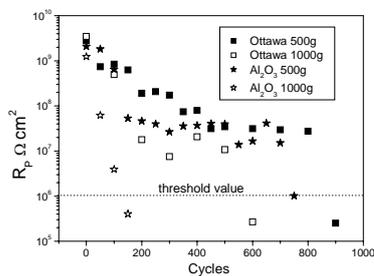
Fig. 3  $R_p$  as a function of Taber Test cycles.
