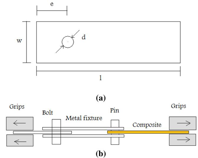
**Fig.1** The schematic view of specimen geometry (a) and testing set-up (b).
