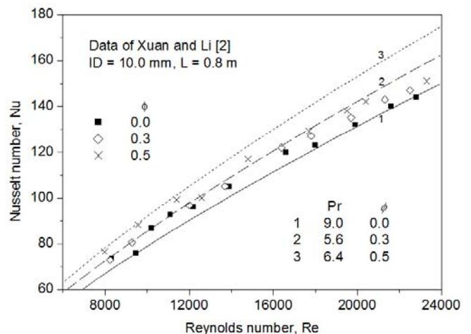
Figure 2 Comparison of experimental values with theory for different values of Prandtl number and  $\phi < 0.5$
