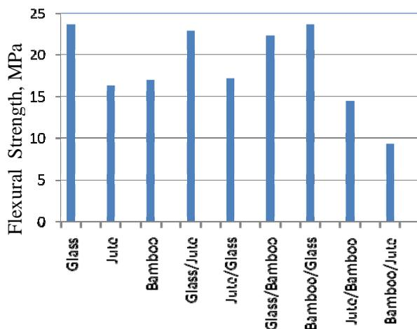
**Fig. 3 Flexural strength of different fiber skinned sandwich structures**
