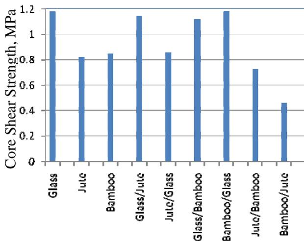
**Fig. 2 Core shear strength of different fiber skinned sandwich structures**
