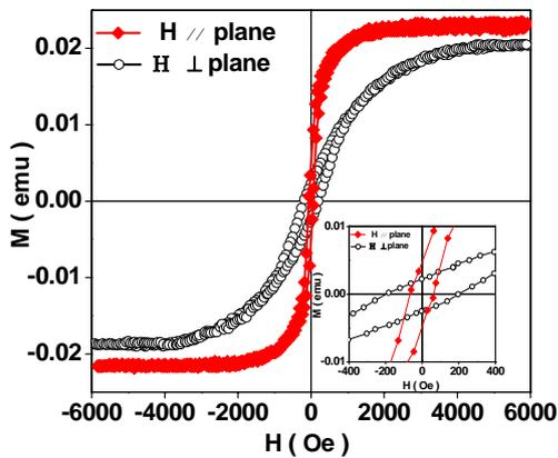
Fig. 2 Room temperature  $M$ - $H$  hysteresis loops recorded with the  $H$  applied parallel and perpendicular to  $\text{Fe}_3\text{O}_4$  film surface. The Inset shows the expanded curve near the origin.
