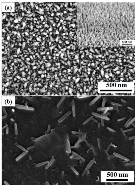
Fig. 1 SEM images of the undoped ZnO and ZnO:Al nanostructures.
