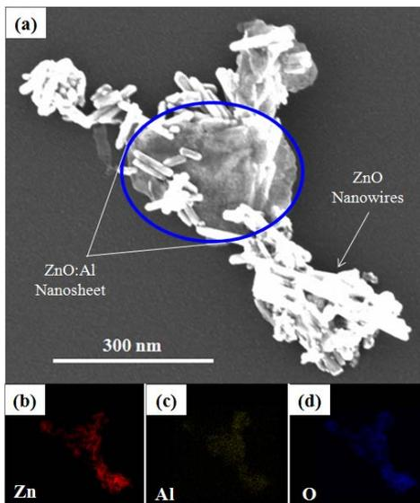
Fig. 2 (a) High magnification SEM image of the ZnO nanosheet doped with 1.0 at.% Al; (b)-(d) Elemental mapping of Zn, Al, and O in a ZnO:Al nanosheet.
