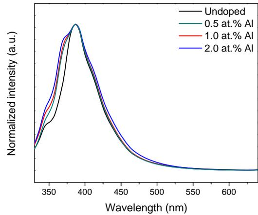
Fig. 3 Normalized room temperature PL spectra of the undoped ZnO and ZnO:Al nanostructures.
