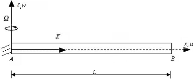
Fig. 1 Schematics of a rotating beam
