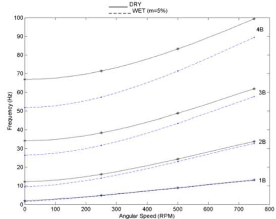
Fig. 3 Rotating natural frequencies of composite beam,  $[15]_{24}$ ,  $T=90^\circ\text{C}$
