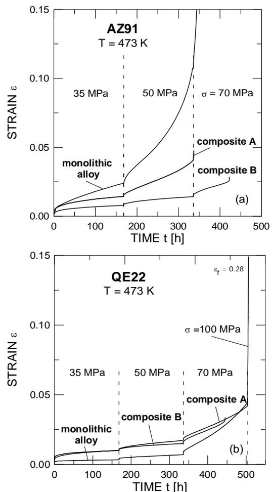
Fig. 1 Creep curves for: (a) the AZ91 alloy and their hybrid composites; and (b) the QE22 alloy and their hybrid composites.
