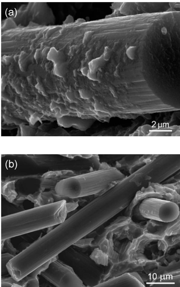
Fig. 2 SEM microfractographs showing carbon fibre surface after creep: (a) composite A – AZ91, (b) composite A – QE22.
