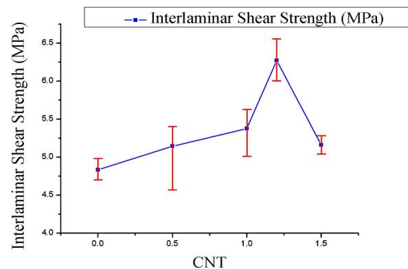
Fig. 2 Effect of CNT on ILSS of C/C composite.
