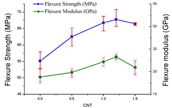
Fig. 1 Effect of CNT content on strength and modulus of C/C composite.
