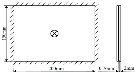
Fig. 1 PVB laminated glazing specimen
