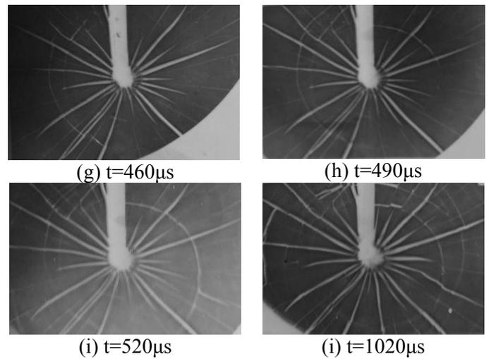
Fig.4 Propagation of cracks
