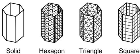
Figure 1. Solid wall and various truss wall honeycombs.
