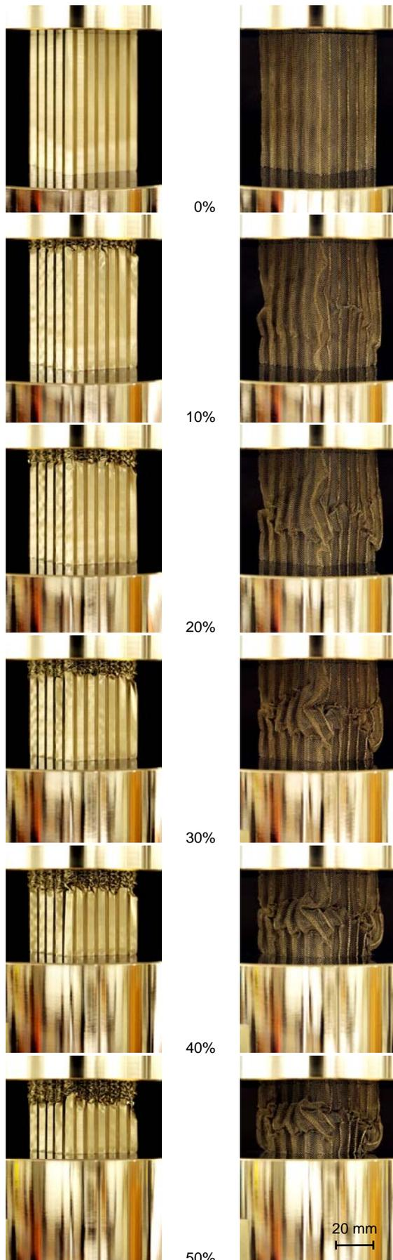
Figure 3. Crushing behavior for solid wall (left) and truss wall (right) honeycombs. Slight outer layer delaminations (right).
