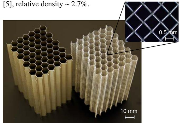
Figure 2. Solid wall (left) and truss wall (right) honeycomb test samples. Microscopic view of a porous truss wall (upper right).
