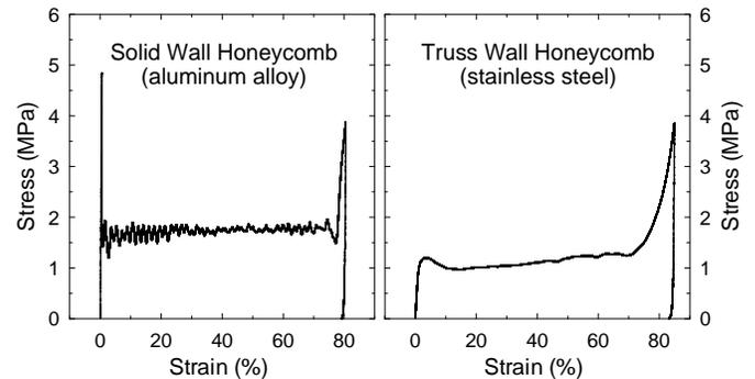
Figure 4. Stress-strain behavior for crushed solid wall (left) and truss wall (right) honeycombs.
