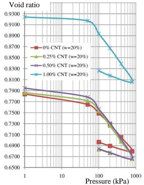
Fig. 2 Consolidation test results at water content (w) 20% for various CNT %
