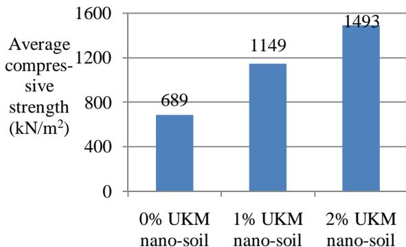
Fig.1 Compressive strength of soil - cement-nanosil mixtures [2]
