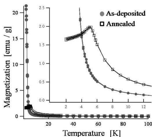
Fig. 1 Temperature dependence of magnetization for the as-deposited (closed circles) and annealed (open squares)  $\text{EuTiO}_3$  thin films under  $H_{\text{dc}} = 100$  Oe applied along the  $\langle 100 \rangle$  direction [6].
