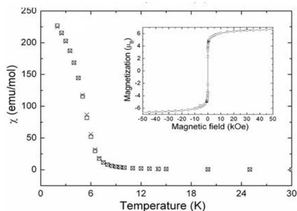
Fig.2 Temperature dependence of susceptibility for amorphous  $\text{EuTiO}_3$  thin film. The measurement was carried out at an external magnetic field of 100 Oe. The crosses and open squares stands for the field-cooled and zero-field-cooled processes, respectively. The inset denotes magnetic field dependence of magnetization at 2 K (open squares) and a guide for the eye (solid line).
