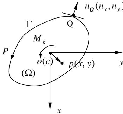
Fig.1 general cross-section of a torsion cylinder
