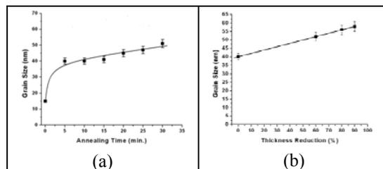
Fig.2 Grain growth kinetics of 46 hours milled Ni-Fe powder during (a) sintering and (b) hot rolling, at 1140 °C
