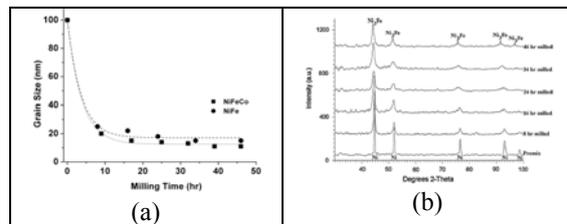
Fig.1 (a) Grain refinement and (b) phase evolution, during mechanical alloying of Ni-Fe and Ni-Fe-Co powder mixture
