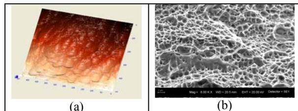
Fig.3 (a) AFM image and (b) fractograph, of bulk NC Ni-Fe strip
