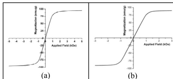
Figure4. Hysteresis curves of bulk NC (a) Ni-Fe (b) Ni-Fe-Co
