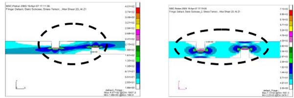
Fig 8- shear stress for UD-45° Fig 9- stress results for UD-90° The results show that FE model prediction of the high stress paths is similar to the failure paths resulting from in plane shear test. It can be concluded that the compression type failure during the in-plane shear test is due to the indentation of 90° plies.
