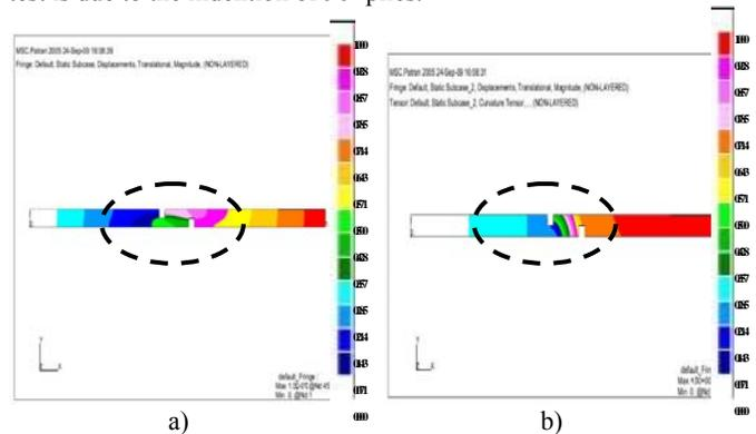
a) UD-45° Failure in shear b) UD-90° failure in compression
