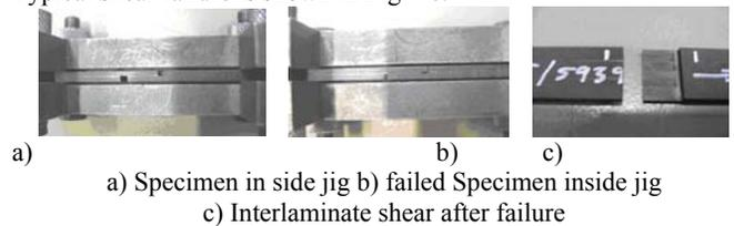
Fig4- typical specimens before and after testing
