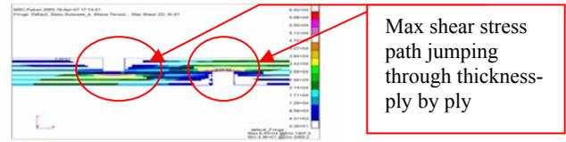
Fig7-the shear stress plot for 45/90 compression failure
