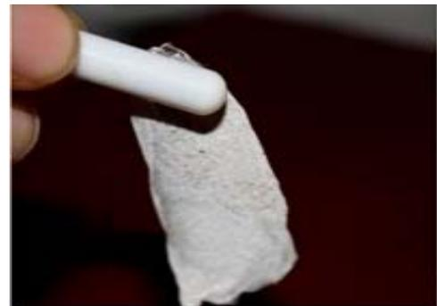
Figure 5 PVdF web attracted by a lab magnet
