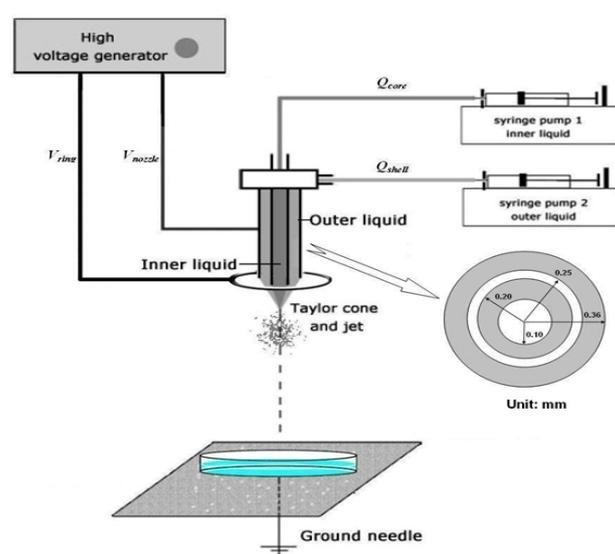
**Figure 1:** Schematic diagrams depicting the set-up of coaxial electrohydrodynamic atomization (CEHDA).  $V_{nozzle}$  and  $V_{ring}$  are 6.5 KV and 3.5 KV respectively in a typical fabrication.
