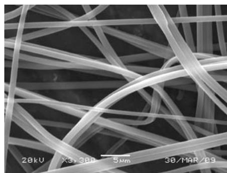
Fig. 2: SEM of Melt Electrospun PP from Trial 4
