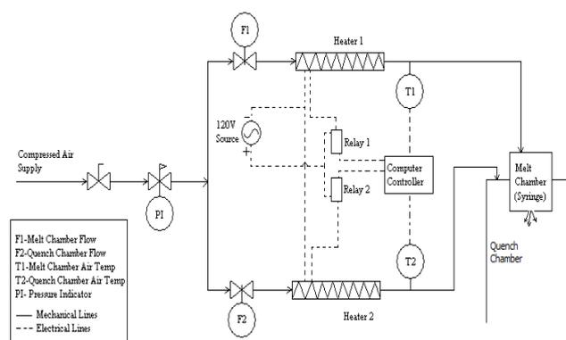
Fig. 1: Piping and Instrumentation Diagram [14]
