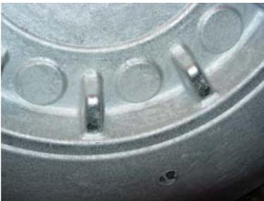
**Figure 6 Rotor with Modified Si Content Showing No Hot Tearing**
