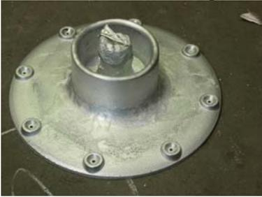
**Figure 4 Sample Castings Poured From Composite**
