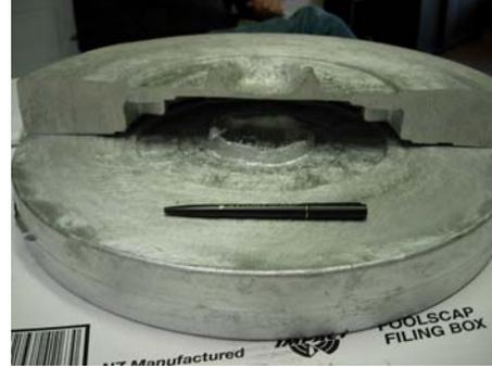
**Figure 1 Rotor Showing Section Differences (6061 Material)**
