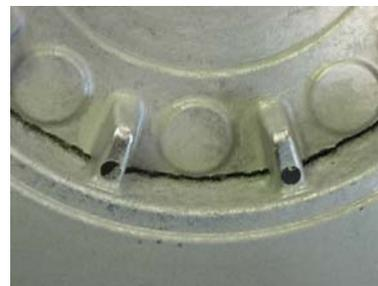
**Figure 3 Composite Rotor Showing Hot Tearing**
