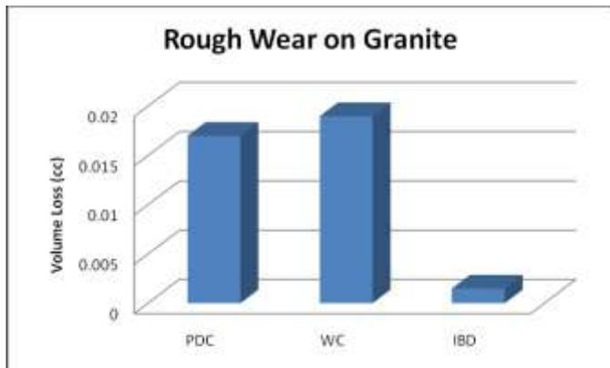
Figure 3. Results of rough wear on granite
