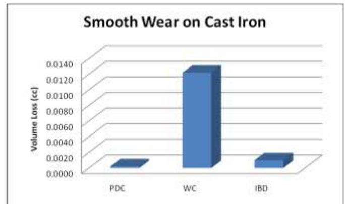
Figure 4. Results of smooth wear on cast iron
